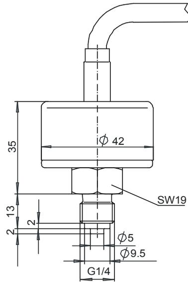
Screw-in aperture according to EN 837
